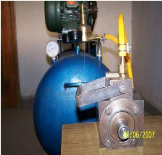
Fig. 4 Compressed Air Turbine –Model under Test
