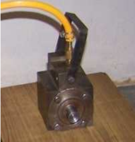
Fig. 3 Compressed Air Turbine –Working Model
