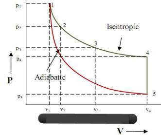
**Fig.6** Polytropic cycle for Air Turbine
