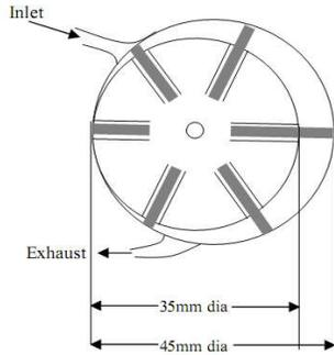
**Fig. 5** Air Turbine –Concept & Cycle
